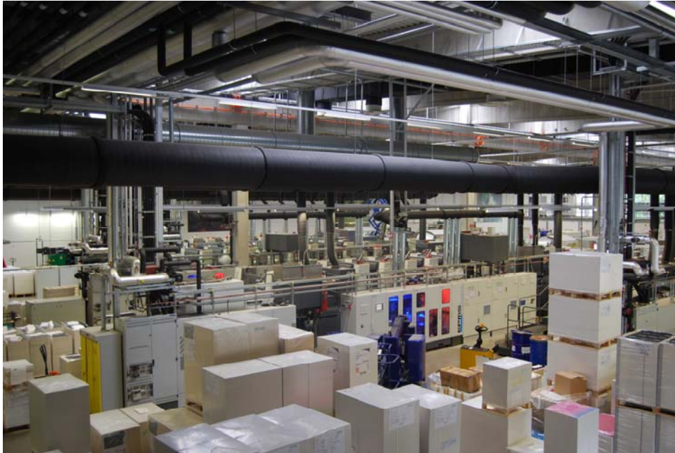
Image 3: The drying units for all printing machines are integrated into the heat recovery system
