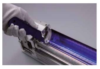
The lamp is removed from the housing and taken out of the unit using the tool supplied.
