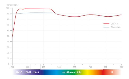
The URS® A reflector has much higher reflectance in the UV range than conventional aluminium reflectors. In the IR range (heat radiation), the reflective properties of the two types of reflector are virtually identical.
