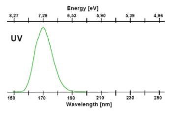
Irradiation with excimer lamps is also suitable for mattifying surfaces such as PVC flooring. At a wavelength of 172 nanometres, these lamps have immensely high-energy emission which starts a polymerization process in the top part of the layer of UV-curable coating. The penetration depth of UV radiation is comparatively low, with the result that this process leaves a micro-folded film on the wet coating without affecting layers deeper down.
