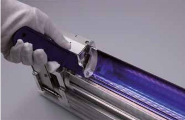
The lamp is removed from the housing and taken out of the unit using the tool supplied.
